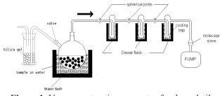
Figure 1. Vacuum extraction apparatus for the volatile compounds in mushrooms
